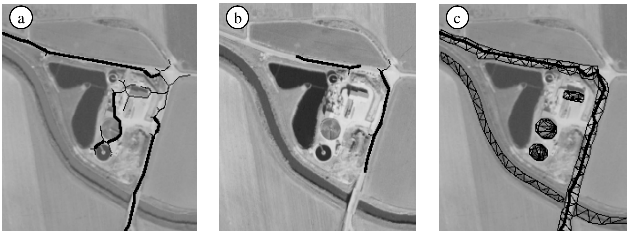
Fig. 2: Rejected (thin line) and accepted (wide line) road features from a) visual and b) infrared image with c) fusion result. Each object (road, river, building, sedimentation tank) is approximated by a polygon mesh to model geometry.
