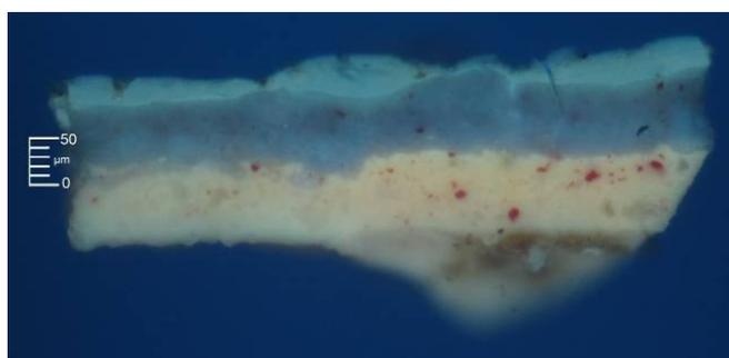
Figure 10 – Cross-section of a micro fragment observed under the optical microscope using an UV lamp.
