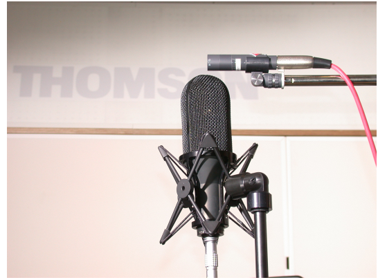
Figure 3: The measurement setup. Above the Soundfield microphone (DSF-1) a measurement microphone (Neumann KM100) is positioned.
