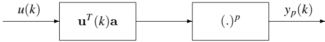
FIGURE 1 – Realization of the p^{th} -order homogeneous term of a Volterra model as a Wiener model. Case of a rank-one kernel.
