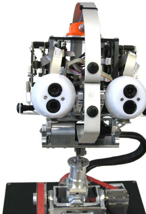
Figure 3: Front view of the head of the humanoid robot ARMAR III.
