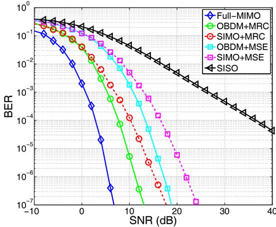
Figure 5: BER performance of the evaluated schemes with time precoding.
