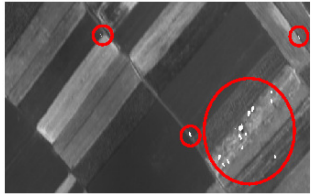
Figure 1: 30th band of a hyperspectral image cube with anomalies marked in white and encircled by red ellipses.
