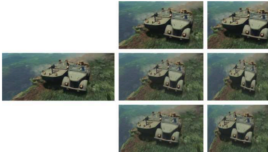
Figure 9: Retargeting of a movie clip (“Indiana Jones” ©2008 Paramount). The original clip in the left side has an aspect ratio 2.38:1. It is resized to the aspect ratios of 16:9 and 4:3, respectively. From top to bottom, the cropping method, the scaling method, and the proposed algorithm.
