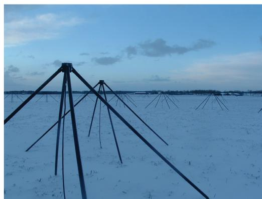
Figure 1: antennas of a low frequency radio telescope (LOFAR) station. The signals are combined by phased array beamforming and correlated with other LOFAR station signals. Sky images are produced by inverse Fourier transforming the correlation products.
