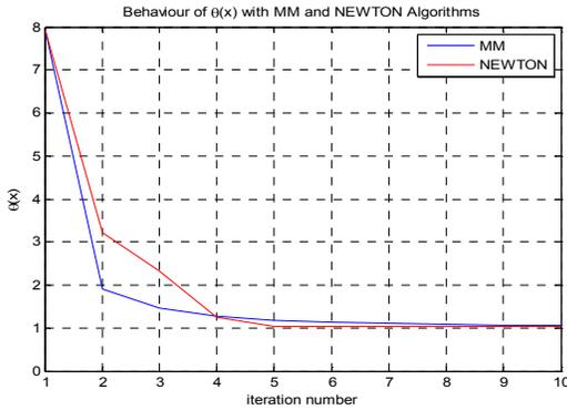
Figure 2 –  $\theta(x)$  versus iteration number of MM and Newton.
