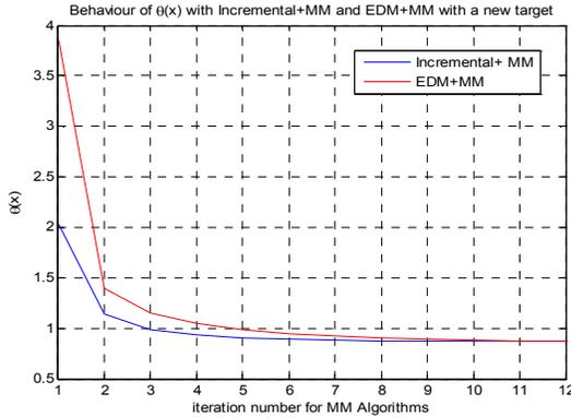
Figure 6—  $\theta(x)$  versus iteration number of MM for EDM-MM and Incremental-MM approaches (1<sup>st</sup> target position).
