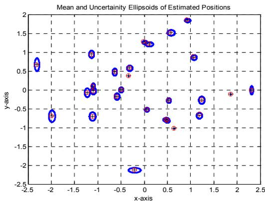
Figure 3 – Calculated mean and variance of estimated positions. The red circles are the real positions of sensors and target. The black + is the mean of the positions and the blue ellipsoids show the uncertainty around the mean values.
