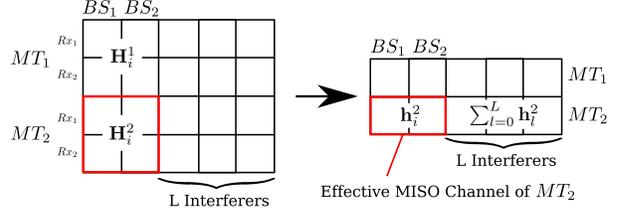
Figure 3: Transforming a MIMO channel into an effective MISO channel with known SINR.
