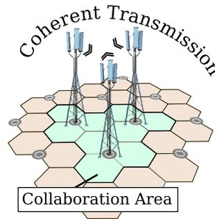
Figure 1: Coherent transmission of collaborative base stations
