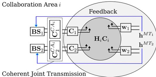
Figure 2: True and effective multi-cell channel. The pre-coder for coherent joint transmission is distributively calculated, while the corresponding parts are used at each of the collaborating BSs.
