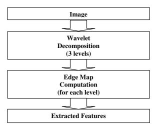
Figure 2 – The features extraction stage.
