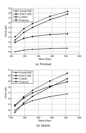
Figure 3: Rate distortion curves for different methods for (a) Foreman sequence (b) Mobile sequence with QCIF size and 15 fps with packet loss rate of 10%.
