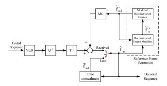
Figure 2: Block diagram of a video decoder with reference frame modification.
