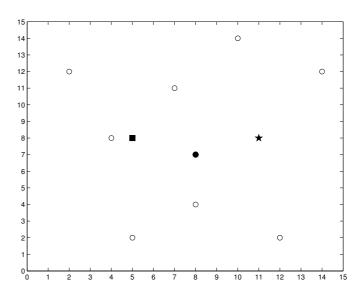
Figure 1: Simulated room scenario with a speech source  $\bigstar$ , a white noise source  $\blacksquare$ , a fusion center with reference microphone  $\bullet$ , and 8 single microphone nodes  $\circ$ .
