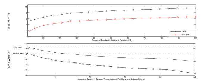
Figure 2: The top subplot shows both the SER and IWSNR as a function of  $\mathbf{B_s}$ . The bottom plot shows the difference between using a full signal and a subset of the signal while varying the time between full  $t_f$  and partial transmission  $t_s$ .
