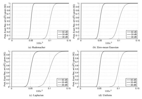
Fig. 2. Best case scenario probability of exact recovery by  $(\epsilon^2 C)$  given (SC), as a function of  $\epsilon^2$  (s=400) for measurements in zero-mean Gaussian white noise at three signal to noise ratios  $(\sigma_y^2/\sigma_v^2)$ , legend) distributed in four ways. Empirical results in (c, d) are averaged over 1000 trials.
