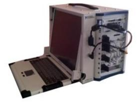
Fig. 2. Mobile eavesdropping system
