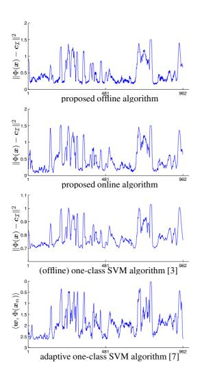
**Fig. 3**. The decision functions estimated by several algorithms. A threshold can be introduced for novelty detection (not illustrated here).
