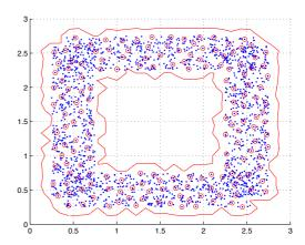
**Fig. 1**. The online method applied on the "frame" distribution. Samples are given in dots ·, and elements of the dictionary are shown with circles o. The contour is given by the distance to the estimated center.
