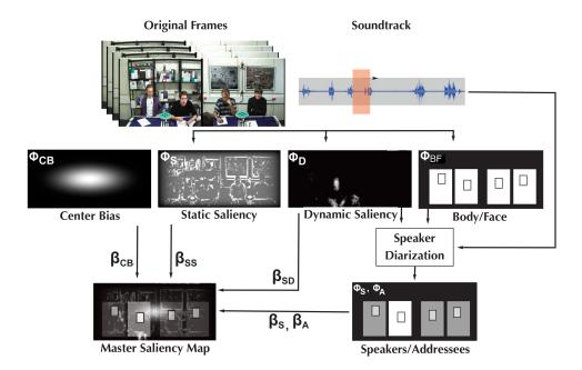
**Fig. 1**. Block diagram of our audiovisual saliency model. Center Bias, Static and Dynamic Saliency, Speakers and Addresses (Faces or Bodies) maps are weighted with the  $\beta^{Lasso}$  estimated weights, and merged into the audiovisual Master Saliency map.
