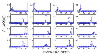
Fig. 2. Paraunitary matrix truncated with  $\mu = 10^{-4}$  using the state-of-the-art approach in [12].
