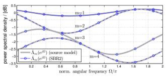
Fig. 1. Power spectral densities of the source model D(z) and of the extracted matrix  $\hat{D}(z)$  using SBR2.
