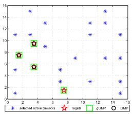
(b) Targets positions estimation when SNR= 10 dB when N=64, K=4, M=20 and q=2.
