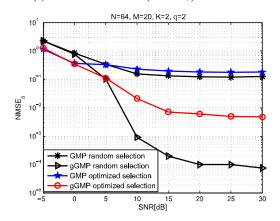
(g) NMSE on cell positions detection versus SNR.
