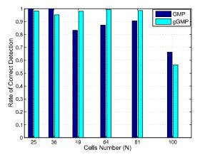
(c) Correct events position detection versus cells number when  $M/N \approx 0.3$ ,  $K/N \approx 0.03$ , q = 2 and SNR= 20dB.
