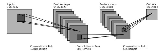
Fig. 1. Architecture of the proposed convolutional neural network. On the upper part are reported the size of the input, intermediary images and outputs. On the lower part the parameters and size of the filters for each layer.
