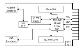
Fig. 1. Block diagram of TMS320C6678 evaluation board
