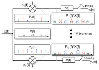
Fig. 1: Sensing process of the MWC.
