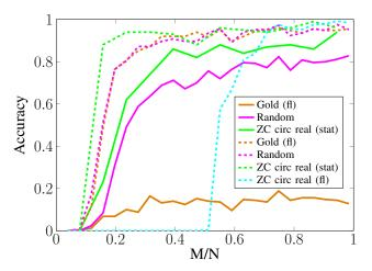
Fig. 5: Accuracy of the MWC with growing compression rate (K=6, 200 trials, OMP reconstruction algorithm), solid:10 dB ISNR, dashed: noiseless.
