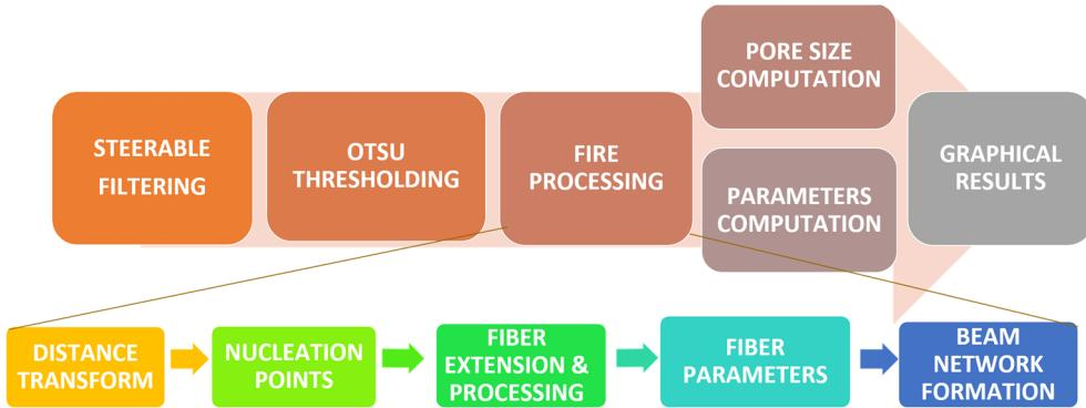
Fig. 4. Schematic workflow of the pipeline. The output of the Otsu thresholding is the binarized collagen network. The main steps of the FIRE algorithm are summarized in the second row. The output of the FIRE processing gives the individual fiber reconstructions, which are used to compute the parameters that characterize the network geometry including the pore size. In a final step, the results are graphically displayed.
