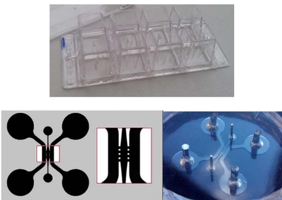
Fig. 1. (Top) Eight-well culture plate; (Bottom, Left) Schema of the microfluidic device. It consists of two lateral channels connected to a central chamber where the hydrogel is loaded; (Bottom, Right) Central chamber and lateral channels in detail.
