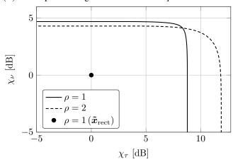
Fig. 1. Pareto regions for bandwidths  $B=\rho f_s$  with  $f_s=10 \mathrm{MHz}$
