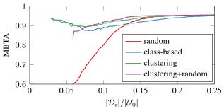
Fig. 7. MBTA of margin sampling with  $N_L=1$  on phase B of BLUED against the ratio of the size of the current training set  $\mathcal{D}_i$  against the number of all available training samples for different methods to select the initial training set.
