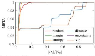
Fig. 5. MBTA of all query strategies without density weighting on BLUED phase A against the ratio of the size of the current training set  $\mathcal{D}_i$  against the number of all available training samples. The initial training set is created by the combination of cluster-based and random selection.  $N_L$  is chosen as 1 for all strategies.
