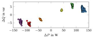
Fig. 3. Clustering of the events of a refrigerator resulting in six clusters.
