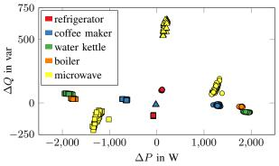
Fig. 4. All samples of the ISS kitchen dataset in the  $\Delta P$ - $\Delta Q$  plane. Circles mark the switching on events of an appliance, squares mark the switching off events. Other state changes are marked with a triangle.
