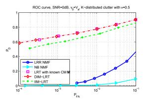
Figure 3. ROC curves for migrating target  $v=v_a$ , SCR=0 dB in K-distributed clutter  $\nu=0.5$ , strongly correlated over range  $\gamma=1$
