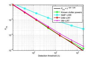
Figure 2. False alarm regulation in clutter strongly correlated over range  $\gamma=1;$  K-distributed clutter  $\nu=0.5$
