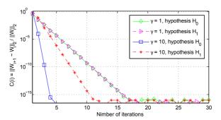
Figure 1. Convergence of iterative estimation in K-distributed clutter  $\nu=0.5$ :  $\gamma=1$  corresponds to strongly correlated over range clutter;  $\gamma=10$  to clutter slightly correlated over range
