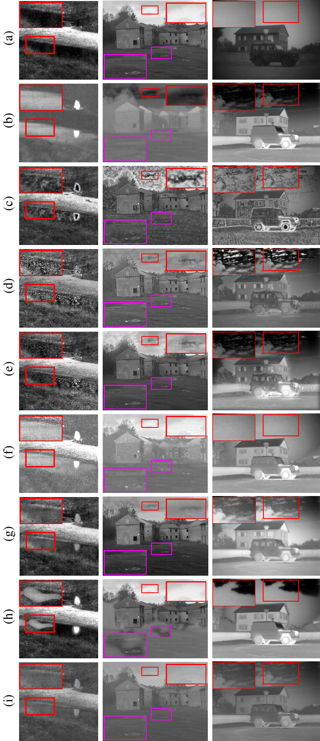
Fig. 2: Visual analysis of results on the Bench, Octec, and Marne image (from left to right). From top to bottom: (a) Visible images, (b) IR images, results of (c) CBF, (d) RP, (e) RP-SR, (f) Fuzzy edge, (g) RFN, (h) DNN and (i) Proposed schemes, respectively.
