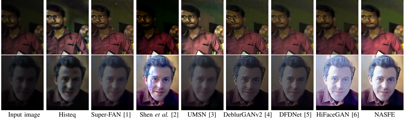
Fig. 4: Qualitative comparisons using real face images multiple degradations collected from YouTube videos. output images of Histeq are computed using Histogram equalization method.
