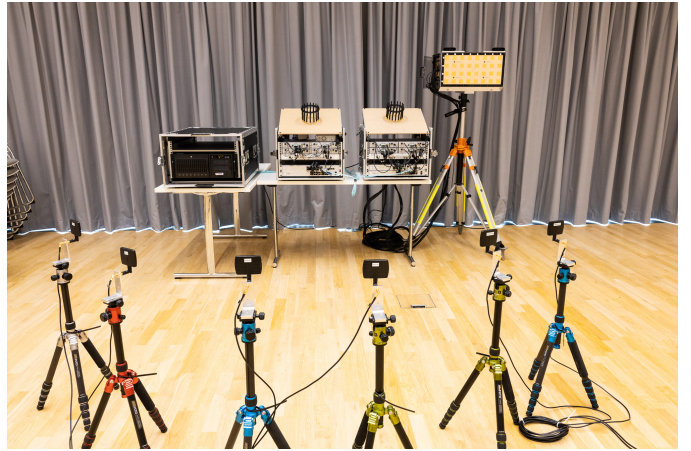
Fig. 2. System setup. The antennas in the front are used as transmitters, the receiver consists of one the circular antenna array in the background (only one is used for these experiments), the Ettus SDRs below it and the server to the left of it.
