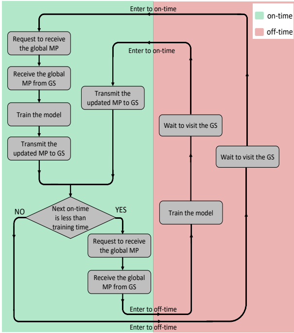
Fig. 4. Flow chart of FedSatSchedule algorithm, the red and green colors represent the off-time and on-time intervals, respectively. MP stands for model parameters.
