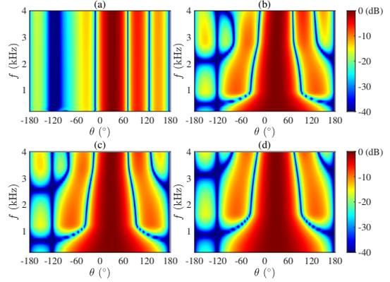
**Fig. 3.** Broadband beampatterns corresponding to the MDF and the proposed robust differential beamformers with a UCMA for different values of  $\mathcal{W}_0$ : (a) the MDF beamformer, (b) the proposed,  $\mathcal{W}_0 = -30$  dB, (c) the proposed,  $\mathcal{W}_0 = -25$  dB, and (d) the proposed,  $\mathcal{W}_0 = -20$  dB. Conditions:  $M = 8$ ,  $r = 1$  cm,  $\theta_s = 30^\circ$ , and  $\theta_1 = 120^\circ$ .
