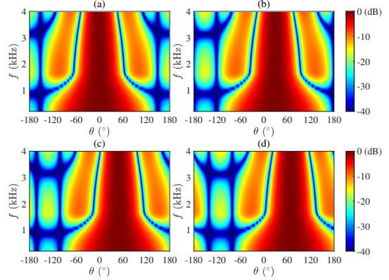
**Fig. 4.** Broadband beampatterns corresponding to the proposed robust differential beamformers based on a UCMA with different steering angles where: (a)  $\theta_s = 0^\circ$ , (b)  $\theta_s = 30^\circ$ , (c)  $\theta_s = 50^\circ$ , and (d)  $\theta_s = 70^\circ$ . Conditions:  $M = 8$ ,  $r = 1$  cm,  $\mathcal{W}_0 = -20$  dB, and  $\theta_1 = 120^\circ$ .
