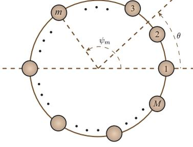
**Fig. 1.** Illustration of a UCMA that has  $M$  sensors, where  $\psi_m$  denotes the azimuth angle of the  $m$ th microphone and  $\theta$  denotes the azimuth angle.
