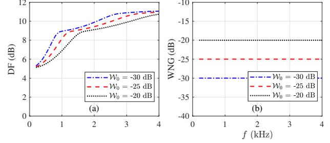
**Fig. 2.** DFs and WNGs of the robust differential beamformer designed with a UCMA: (a) DFs and (b) WNGs. Conditions:  $M = 8$ ,  $r = 1$  cm,  $\theta_s = 30^\circ$ , and  $\theta_1 = 120^\circ$ .
