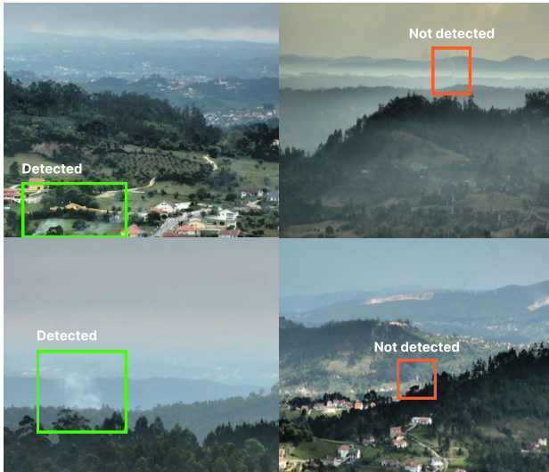
Fig. 4. Examples of predictions by the ensemble model. Left: true positives (green bounding box); right: false negatives (red bounding box). The bounding boxes are simply illustrative to know the position of the fire sign in the image.
