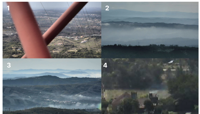
Fig. 1. Example of images taken from cameras mounted in surveillance towers with different types of occurrences hard to predict. 1: Image obstruction. 2: Foggy sky. 3: Low clouds. 4: Chimney smoke.
