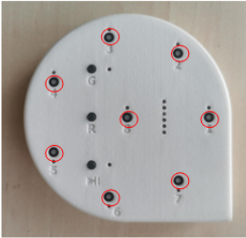
Fig. 2. Recording device. Microphone positions are marked with red circles.
